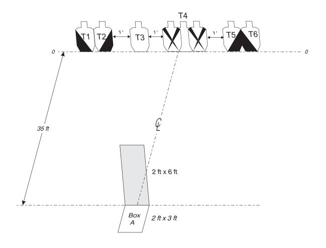
**SETUP NOTES:** Set paper targets to 5 feet high at shoulders. Space paper targets 1 foot apart. Barricade is 2 feet wide and 6 feet high with a 2-feet-by-3-feet
